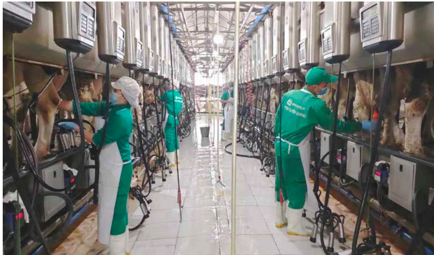
The automatic milking unit which can receive more than 200 cows/milking
